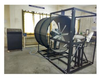
Wind Energy Training System is a miniature replica of actual wind turbine power plant. This system facilitates the researchers with working and configurable model of wind turbine. This system gives the insight about individual components and consequences of changing the operating points of any wind turbine defined in terms of wind speed and pitch angle. researchers can learn concepts like I-V characteristic, cut-off, cut-in speed etc.
